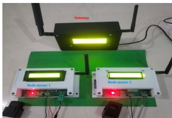
Figure 13. Photo of voltage source monitoring tool
