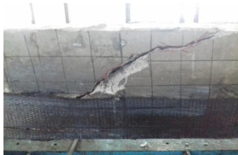
Figure 1. Bending Cracks in Concrete Beams with CFRP Wrap Reinforcement
